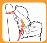
LATCH Strap with Top Tether Strap Do not install with the LATCH system for a child weighing more than 45 lb (20 kg)
