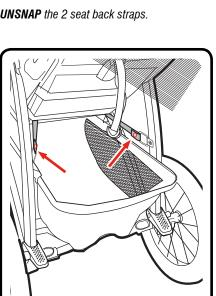
From the right side of the stroller, **SEPARATE** the fold strap as shown **(A)**. From the opposite side, pull the fold strap out of the pocket **(B)**.
