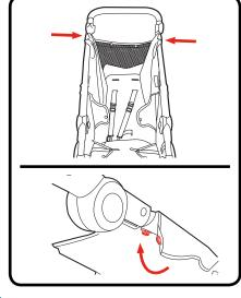
LIFT seat pad, then THREAD the ends of front seat straps through the loops and pull tight. FASTEN the hook and loop tape.
