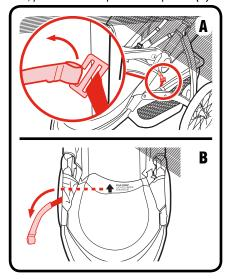
**UNFASTEN** the 12 snaps, and remove the seat from the frame.
