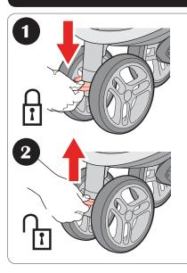
Front swivel wheel lock for use on uneven surfaces such as grass, stones or gravel.
