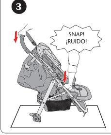
**CHECK** that the stroller is completely latched open every time you open the stroller and before continuing with the rest of the assembly steps. Push down on stroller to be sure seat is locked.
