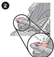
Pull on armbar to be sure it is secure. Open carseat attachment flap as shown.
