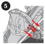
Thread straps through button holes on each side of seat cover.
