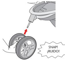
**CHECK** that wheel is securely attached by pulling on wheel assembly.
