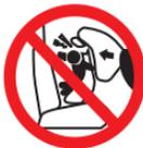
**NEVER place this child restraint rear-facing in a vehicle seating location that has an active front air bag.**
