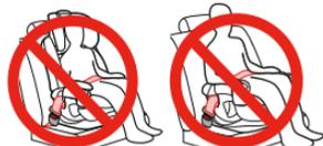
booster mode with vehicle lap belt only seat belt
