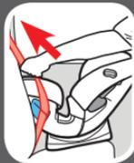
**Note:** When using the lock-off, you do not need to switch the retractor. The lock-off locks the seat belt.
