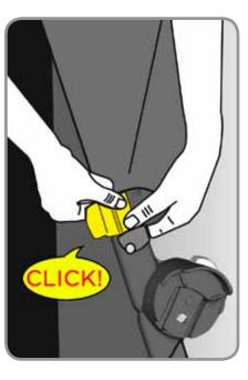
**3** Firmly press the canopy bracket on the seat frame until it clicks into place. Repeat on other side.
