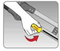
• Pinch gray tabs and pull towards you. Push brake lever down until it is parallel with the frame.
