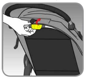
**1** Lift up on flat lever located under the top seat back.
