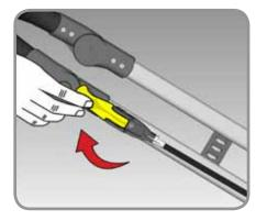
• Pull brake lever into upright position until it clicks into place. Gently push stroller to ensure the brakes are properly engaged.
