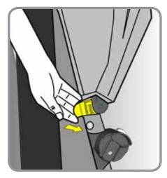
**1** Pull the canopy bracket out and away from the seat frame to detach. Repeat on other side.
