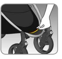
**NOTE:** Be sure the lower front of the basket is placed in the groove of the Versa plate near the bottom of the frame.
