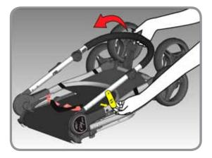
**1** Pull up on the auto-lock to release the frame while lifting up on the stroller handle until the frame clicks into place.
