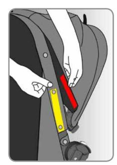
1 Place the rear of the canopy over the top of the seat frame. Secure canopy Velcro® to Velcro® on the seat fabric.
