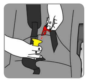
Simply push top right buckle clip into the right side of the center buckle until it clicks into place. Repeat on other side. The buckles should always be clicked into place before using the stroller.
