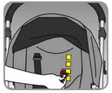
**2** Slide the harness clip out and re-clip to the seat loop closest to the child's shoulder height.
