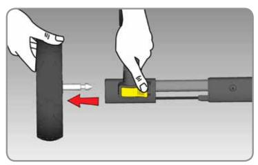
**1** Press the wheel release button while gently sliding the wheel axle out of the wheel mount.
