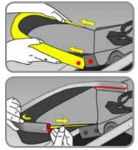
**3** Press gray buttons and pull out on footwell to remove the footwell bar from the seat frame. Pull seat fabric out of channel in footwell bar.
