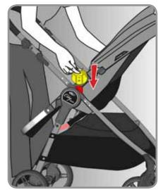
**1** Align seat adaptor brackets with mounting brackets on stroller frame.
