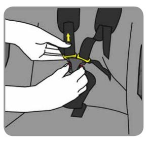
Push one side of the center button and pull the corresponding side buckle clip away from the center buckle. Repeat to unbuckle other side.
