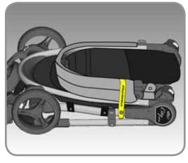
**2** Attach seat storage strap to stroller frame just below the fold mechanism.
