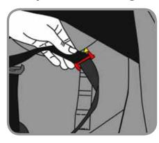
**1** Lift up on the bottom of the harness clip and remove harness strap from the side retainers.
