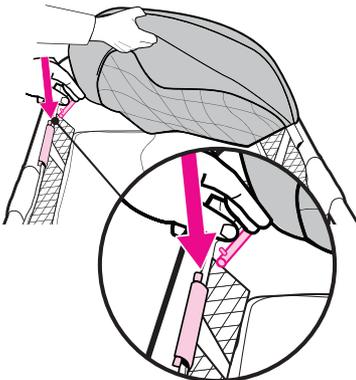
Insert tube into channel on inside of bassinet as shown. Pull open channel for easy insertion.
