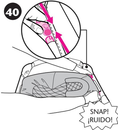
Insert metal tube into plastic tube.
