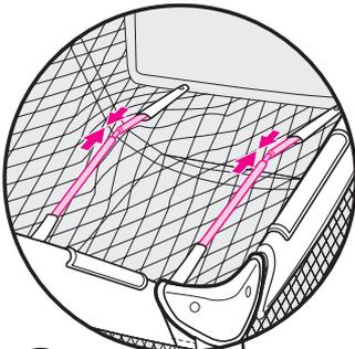
Insert tapered end of bar into end of other bar with hole in it. Repeat with other set of bars.
