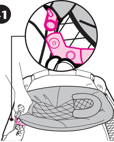
Insert opposite metal tube into plastic tube.
