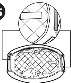
Make sure snap buttons are facing down so that they are not visible from above.
