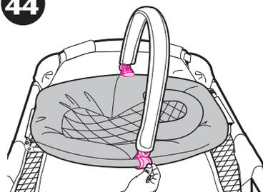
Firmly attach toy bar to napper by clipping the toy bar mounts to the sides of the napper as shown.
