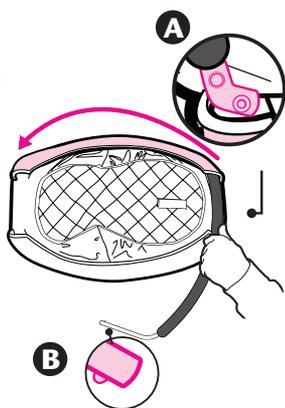
Insert tube with plastic end into channel opening **A**. Snap buttons should be down as shown **B**.
