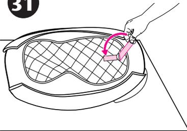
Secure hook and loop tape as shown.
