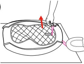
Insert the head support strap through the slot in the napper. **MAKE** sure strap is not twisted.
