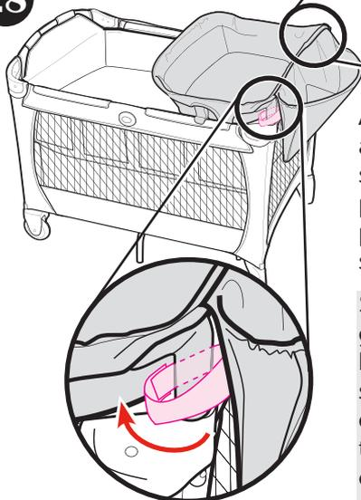
Attach hook and loop straps around posts of changer as shown. Make sure it is properly secured to the playard by pulling up on the sides of the changing table.
