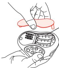
Remove battery door and insert 3 AA (LR06) batteries (not included). Replace door and screws.
