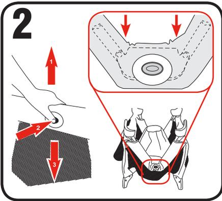
2. Lift rail up slightly, press button and lower rail. Repeat on all 4 sides. (See page 10)
