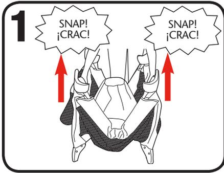
1. Pull up on all 4 sides and snap into place. Do not push center of Playard down until top rails are locked. (See page 7)
