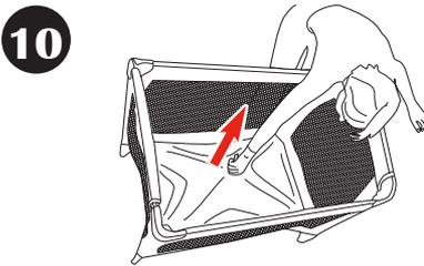
**DO NOT** unlock top rails yet. Center of floor must be halfway up before top rails will unlock.
