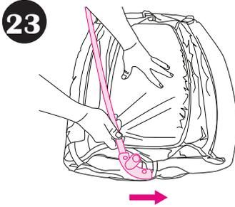
Slide tube through fabric as shown. Repeat with other tube.
