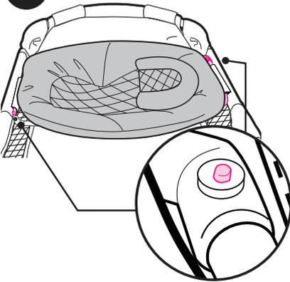
Press buttons on both sides of napper to release metal tubes from plastic tubes.
