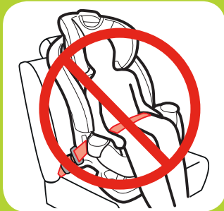
Never use a vehicle lap only seat belt across front of child.
