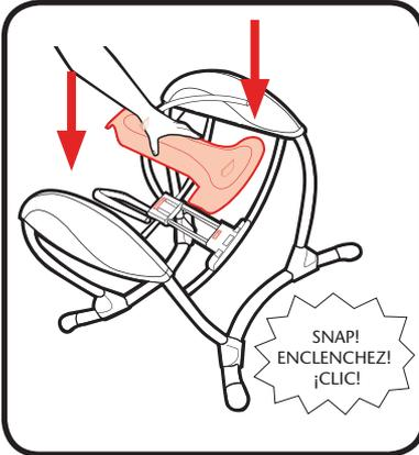
4. Attach plastic cover over tubes as shown until it snaps into place.
