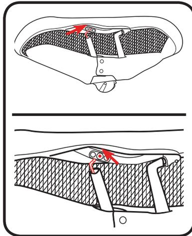
5. Attach hook and loop tape on both sides of seat.
