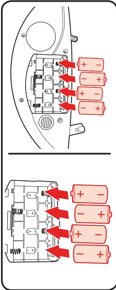
**1. With baby out of swing,** open the battery compartment lid by inserting a key into the slot. Insert four D (LR20 -1.5V) batteries. Replace battery lid.
