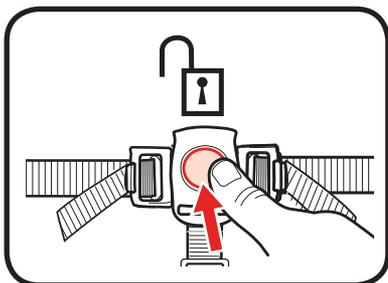
2. To release press button in center of buckle.
