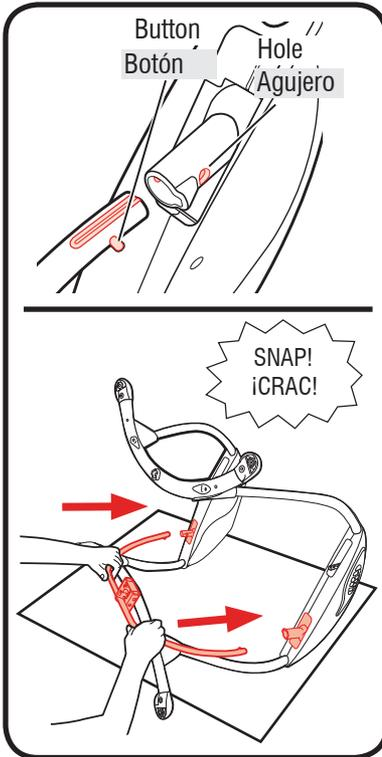
1. Insert the single hinge swing arm into the housing with buttons lining up with the hole in the housing as shown.
