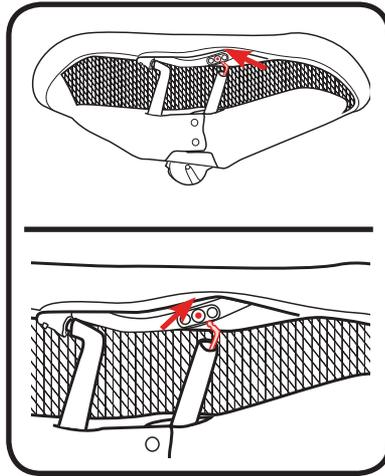
4. Insert side wire on other side of seat into hole in tube as shown.
