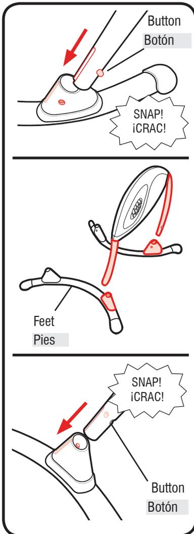
1. Lay feet on floor. Insert battery housing leg tubes into both feet as shown.
