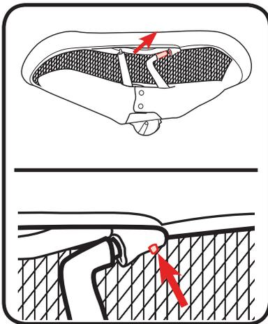
2. Insert side tube on other side of seat into connector on tube as shown. CHECK that button is visible in hole in connector.
