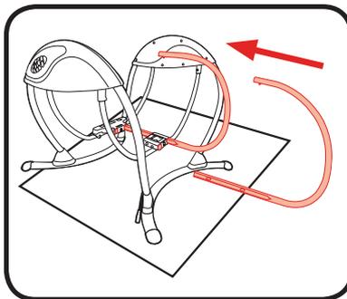
2. Insert the hanger tube with the oval-shaped holes into the swing arm bracket as shown.
