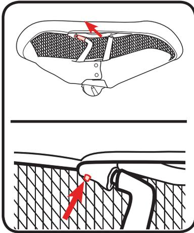
1. Insert side tube of seat into connector on tube as shown. CHECK that button is visible in hole in connector.
