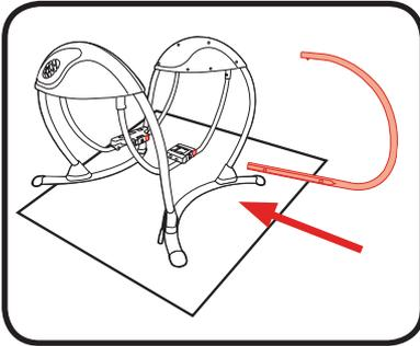
1. Insert the hanger tube with the six-sided holes into the swing arm bracket as shown.
