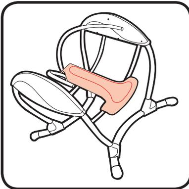
5. CHECK to make sure the cover is attached by pulling up on it.
