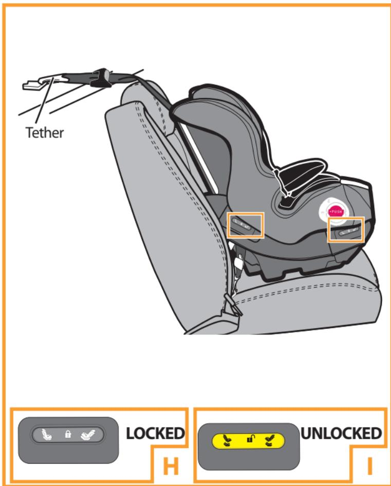
All **LATCH** seating positions have tether anchors. Always use tether if a vehicle tether anchor is available in forward-facing mode with harness. Check your vehicle owner's manual for the tether anchor location(s). If your vehicle is not equipped with a tether anchor, it may be possible to install one. Contact your vehicle dealership for the proper anchor location and installation.
