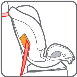
VEHICLE LAP ONLY SEAT BELT WITH TOP TETHER STRAP
