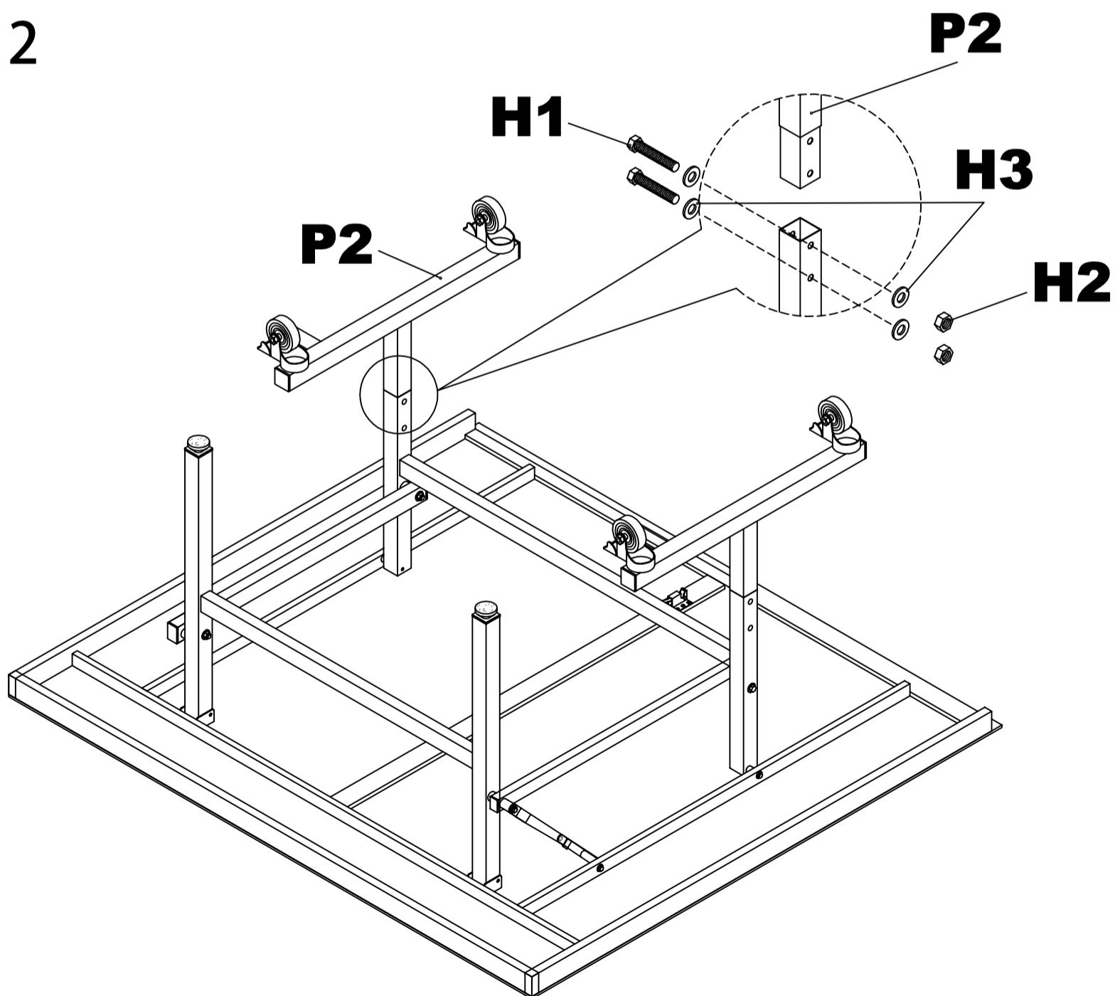
Insert caster feet into table legs, so that holes are aligned. Using wrench, secure feet to legs with provided bolts, washers, and nuts.
