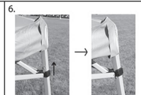
6. Open the canopy frame until all four corners lock into place. You should hear a click when the canopy frame has opened and the corner has locked.
