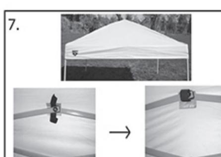
7. Turn all four sides down to cover the side of the frame. On the inside of the canopy, secure all four sides and ceiling to the canopy frame using the inside hook and loop strips.
