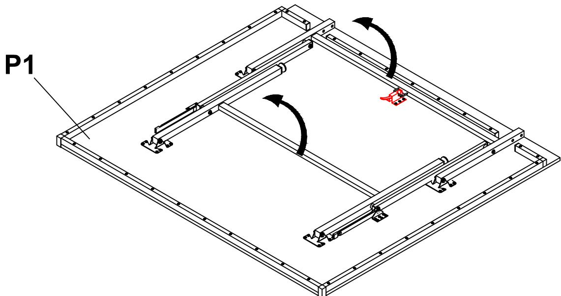
1. Lay tabletop pieces play-surface down on a flat, non-abrasive surface.
