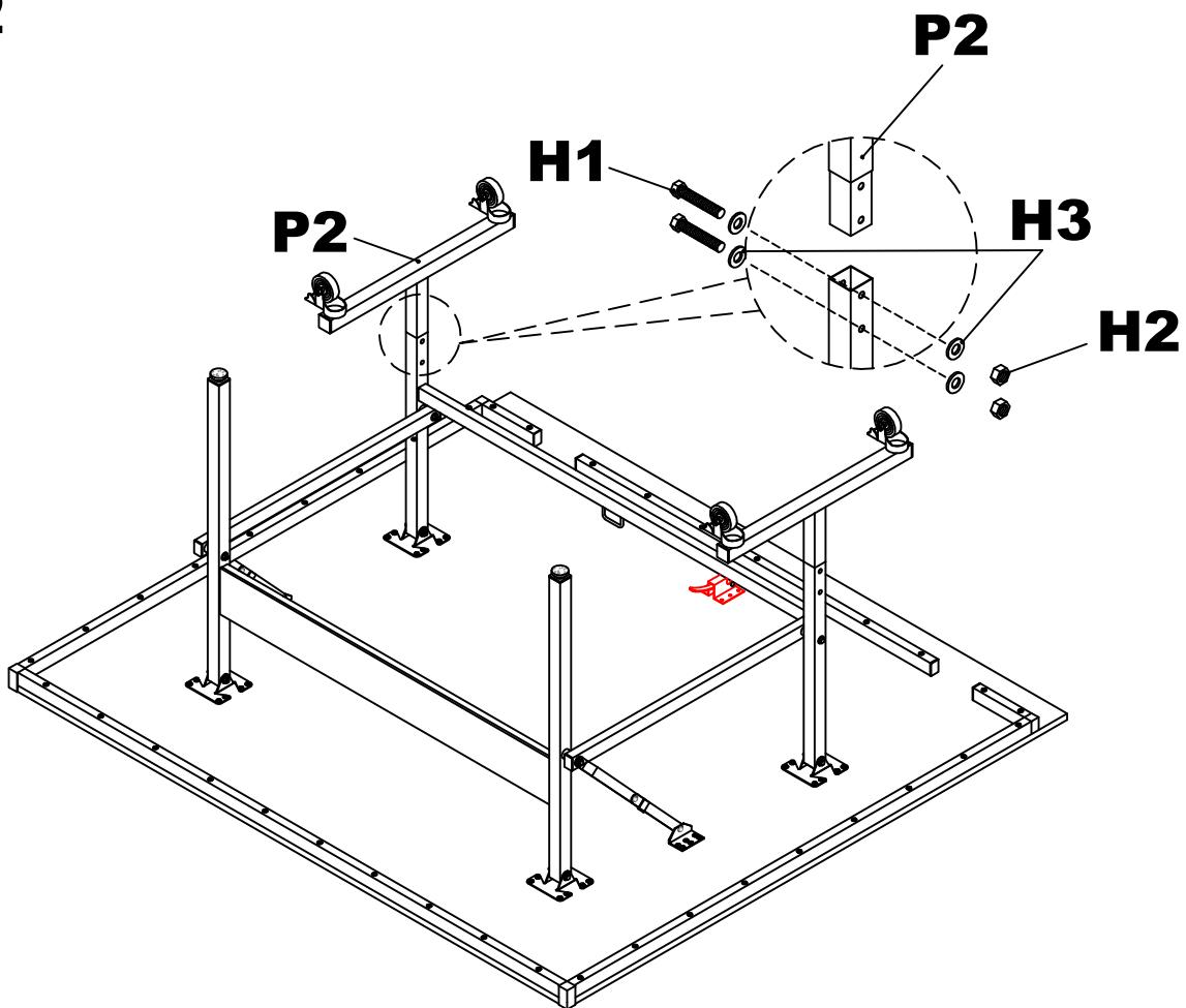
Insert caster feet into table legs, so that holes are aligned. Using wrench, secure feet to legs with provided bolts, washers, and nuts.
