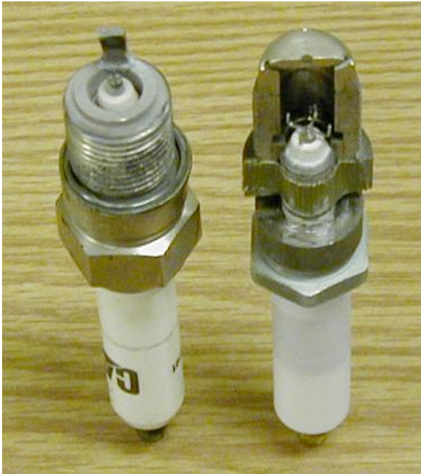
Figure 4: J-Gap (left) Versus Prechamber (right) Spark Plugs
