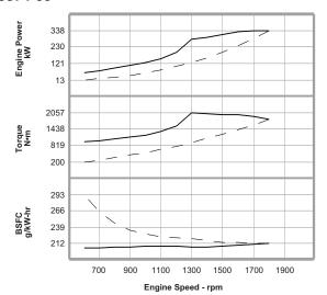
Metric Maximum Power \_\_\_\_\_ 339 kW
