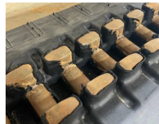
Exposed Embeds (Center Flange Track Rollers)
