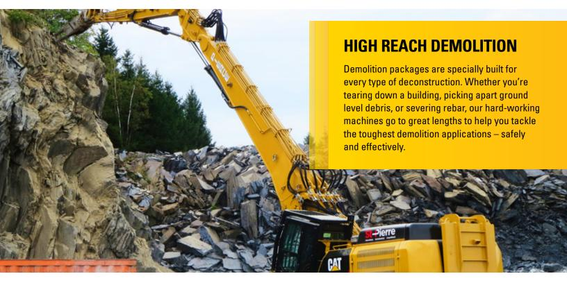
2-piece, intermediate height demolition fronts are ideal for moderate teardowns and demolition, such as sorting, processing, and loading. 3-piece demolition fronts can be customized for multiple heights, ranging from large work tools with impressive production at lower levels to ultra high reach for extremely tall structures.
