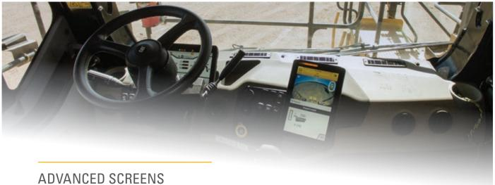
Machine data, controls and guidance information are consolidated onto two 10-inch screens to reduce the number of displays required and present the right information when needed. The screens are ideally located to enable the operator's eyes to remain forward as much
