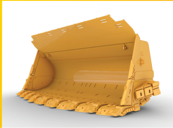
Heavy Duty Rock bucket for the 995 Wheel Loader 24.5 m 3 (32 yd 3 )
