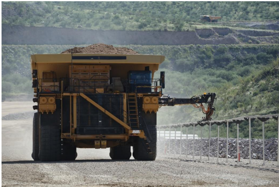
Cat® Dynamic Energy Transfer system prototype under development at Caterpillar Tucson Proving Ground
