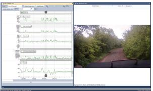
cameras. Resolution, frame rate and other camera settings can be statically configured or dynamically managed by the PowerView recorder based on locomotive operating conditions.
