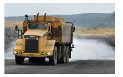
The Haulmax 3900 series off-highway haul trucks are ideal in soft underfoot conditions where superior braking capacity, surefootedness and ground pressure is critical. They offer excellent retardation by dual rear drive axles and eight wheels, delivering greater traction and performance safety.
