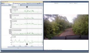
cameras. Resolution, frame rate and other camera settings can be statically configured or dynamically managed by the PowerView recorder based on locomotive operating conditions.
