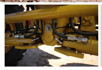
Front axle steering cylinder has been designed to enhance durability and hydraulic hoses have been routed to improve reliability.
