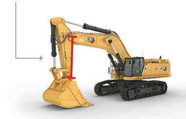
The haulers should position themselves within reach of the excavator's boom, at an angle of no more than  $45^{\circ}$ .
