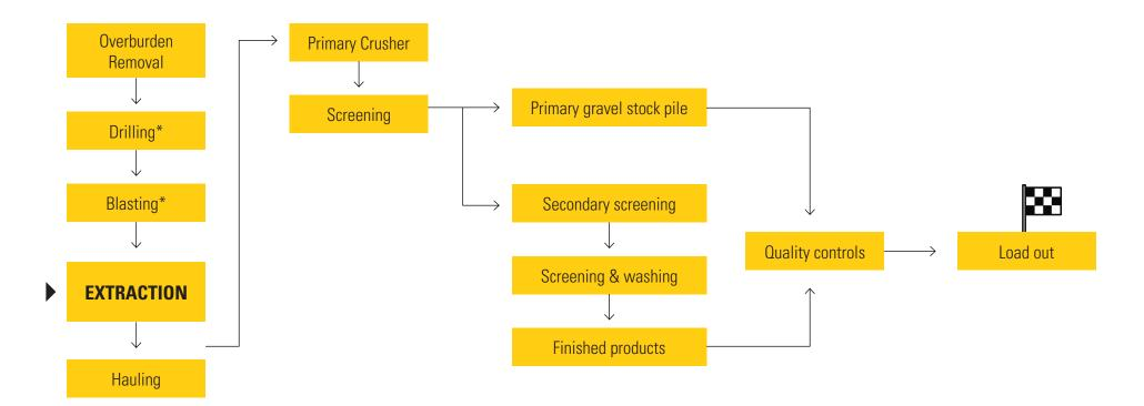
The newly-exposed stone is first loosened by blasting or ripping, loaded into haulers by excavators or wheel loaders, and finally transported to the crusher.
