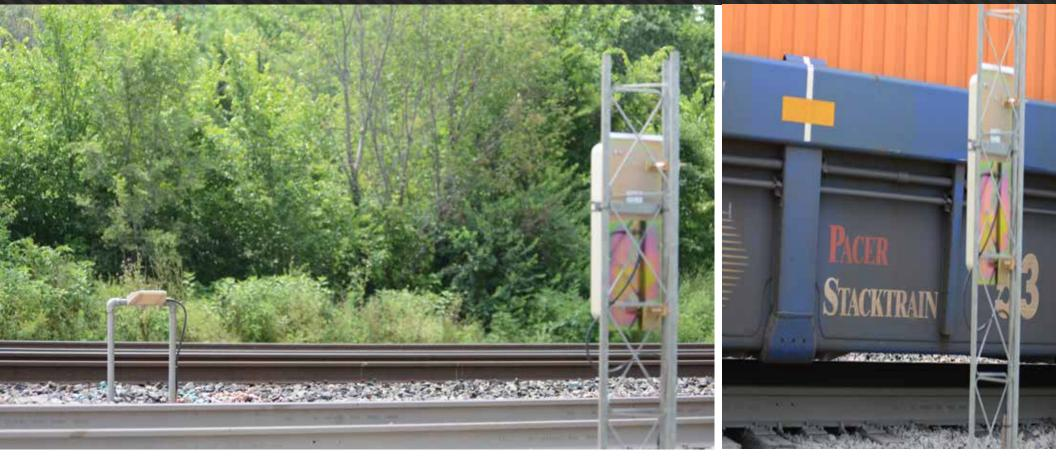
Automatic equipment identification (AEI) is an electronic recognition system. Consisting of passive tags mounted on each side of rolling stock and active trackside readers. AEI uses RF technology to identify railroad equipment while en route. Collected data offers up-to-the-minute tracking on railcars and their location.
