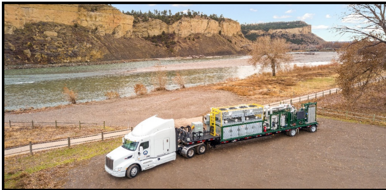
Figure 4: GTUIT's mobile & modular fuel gas processing system
