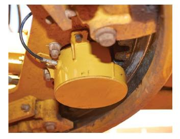
with an aftermarket auto lube system, the Circle Saver attachment enables this maintenance point to be included in the lubrication system.
