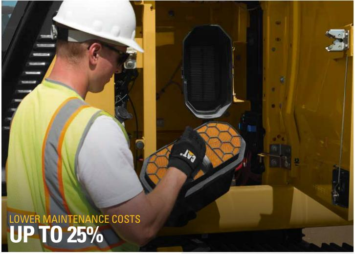
With extended and more synchronized maintenance intervals, you get more done at a lower cost compared to the 320F. Consolidated filter locations make service faster. Hydraulic, air, and fuel tank filters have increased capacity and longer life.
