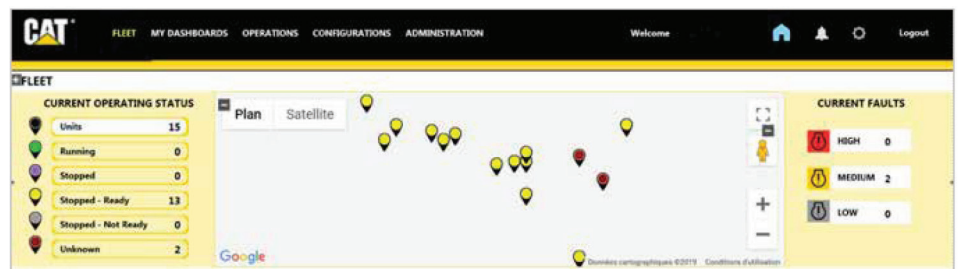
Image: Fleet view in Cat RAM of the 16 connected generator sets
