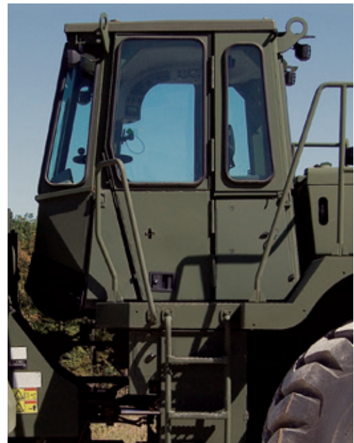
Entry ladder with self-cleaning steps and wide front and rear platforms.
