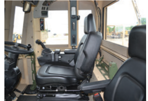
Two-person cab with rifle brackets.
