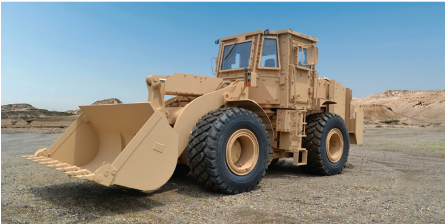
966H fully armored with two-person cab.
