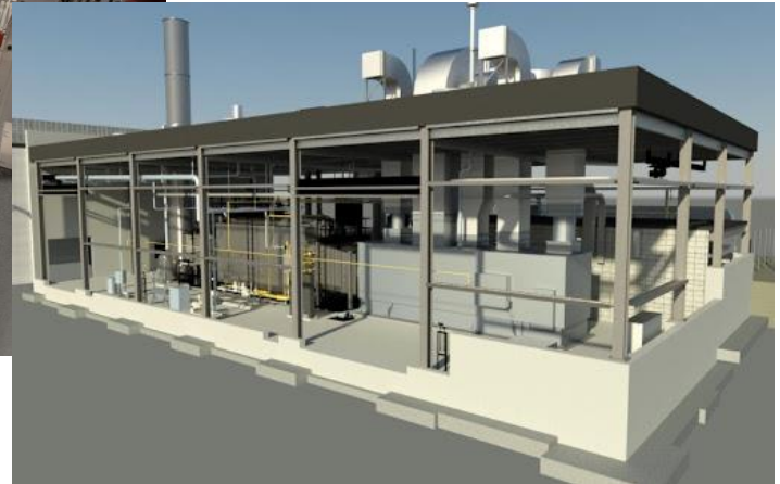
Artist's Cutaway Rendering of the CHP Plant
