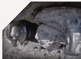
Cat® HDXL with Duralink™: 3,300 hours, 70% rail wear, .24" scalloping.
