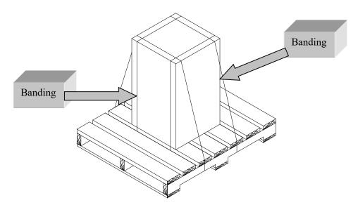
There are numerous options to consider when designing a pallet: the various species of woods available plus the part size and weight. A pallet supplier can assist in determining the correct pallet through the use of a "computer pallet program" that automatically calculates the inputs (part size and weight) and it designs the correct pallet.
