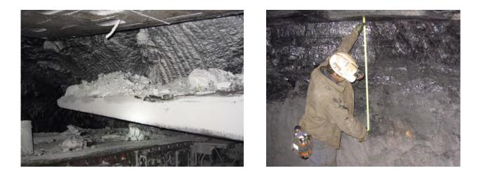
The 7 East face had 5 to 6 ft (1.5 to 1.8 m) of laminated rock interburden above the Blue Creek seam, as well as 4 to 12 in. (10 to 30 cm) of draw rock immediately above the seam. Some areas of the longwall panels had 12 to 40 ft (3.7 to 12.2 m) of sandstone above the seams, which did not always cave as desired after the longwall passes.
