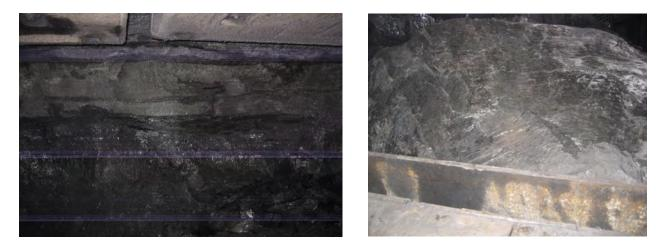
Single-seam mining can be optimal because it eliminates the need to cut, handle and process the middleman rock. However, the payoff depends on the thickness of the thinner Mary Lee seam. When twin-seam mining, more coal is recovered, but mining the rock interburden takes time and increases wear and tear on machinery, including the preparation plant.
