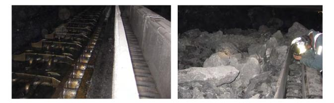
All productive longwalls manage face conveyor chain tension carefully. Too much tension leads to high wear of chains, sprockets, flight bars, pan lines and drive ends. Too little tension leads to slack that can let the chain "tangle" when it goes over the drive sprockets. The result is a chain wreck that can cause many hours and even shifts of downtime.
