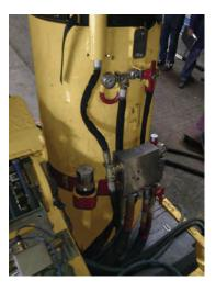
When single-seam mining is done, the primary challenge is to maintain roof control under the middle man. A shield with high density (greater than 10 tons or 9 metric tons per square foot) is typically selected. The roof support must have high capacity at low operating heights to prevent yielding and consequently trapping the shearer.
