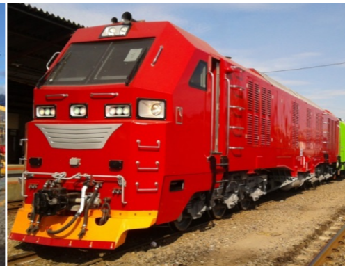
Indonesia loco with 3512B and C15 Head-End Power Package
