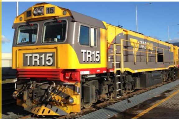
Tasrail loco with 3512C HD and traction alternator package
