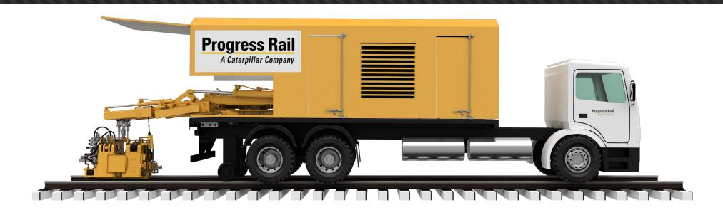
Progress Rail Welding (PRW) offers several Containerized Rail Welding System's one of which is the Model K950 Flash Butt system. This System is Self-contained and fully enclosed, shipped ready for service. The design of the enclosure and base provides for the unit to be mounted as a static plant welder or installed directly on a truck chassis (or flat wagon of a proper height) for mobile operation in-track.
