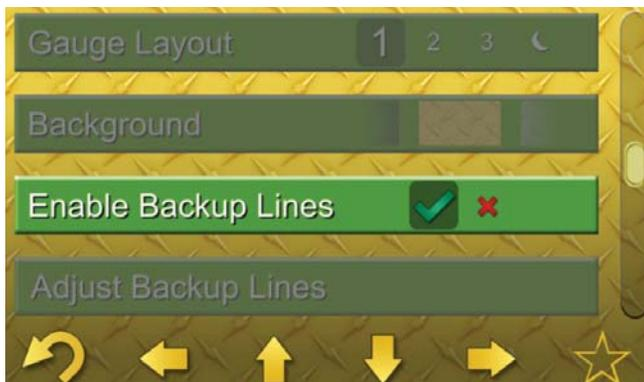
The “Enable Backup Lines Adjustment” allows the operator to turn on reference lines when the display is in Backup Camera Mode. The Machine Width reference lines provide an approximate indication of the backup path of the machine in a straight line. The Rear Distance reference marks provide an approximate gauge of how close objects are to the rear of the machine.
