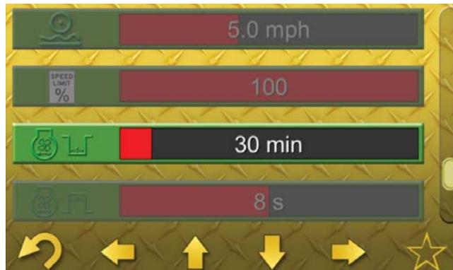
The “Reversing Fan Frequency” is the time between reverse cycles in the automatic mode. The lower the setting, the more frequent the reverse cycle will occur.
