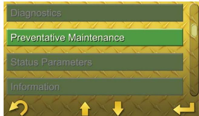
The "Preventative Maintenance" interval screens are pop-up reminders to indicate that a scheduled maintenance interval is approaching. These intervals are based on machine hours and can be reset by the owner after the maintenance is performed. The screens will provide the operator several pieces of information including:
