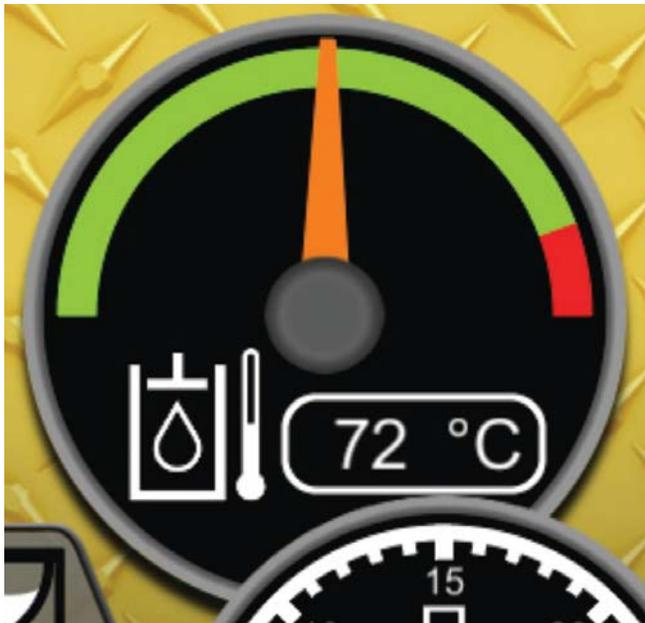
The needle in the red zone indicates that the hydraulic oil temperature is too high. If the gauge's numerical values are enabled, the background will change from black to red to indicate that the hydraulic oil temperature is approaching an unsafe temperature. The hydraulics functions should be stopped soon and the engine set to low idle to allow the hydraulic system to cool. See "Menu Screen, Display Settings, Digital Readout."
