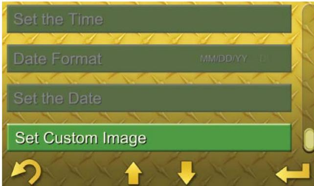
This screen allows the owner to upload a custom image that will be used as the “splash” screen image which is visible while the display boots up after each key ON. The image is loaded via a USB thumb drive plugged into the machine’s USB port. The image must be either a .jpeg, .jpg, or .png file and formatted 800 × 400 for best fit. See “Operator Controls, Left Side Controls, Power Supply Port.”
