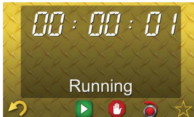
These screens allow the operator to start, stop, and reset a job clock. The job clock saves over the key cycle and starts up automatically on the next startup or operator login. A separate job clock is stored under each operator profile.
