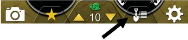
The menu screens for smart attachments are accessed from the Monitoring Screen by pressing the soft key under this icon. The portal to smart attachment screens is only available when the machine ECM detects the presence of a smart attachment via the machine's electrical connector. The smart attachment monitoring and adjustment screens will vary depending on which attachment is connected.
