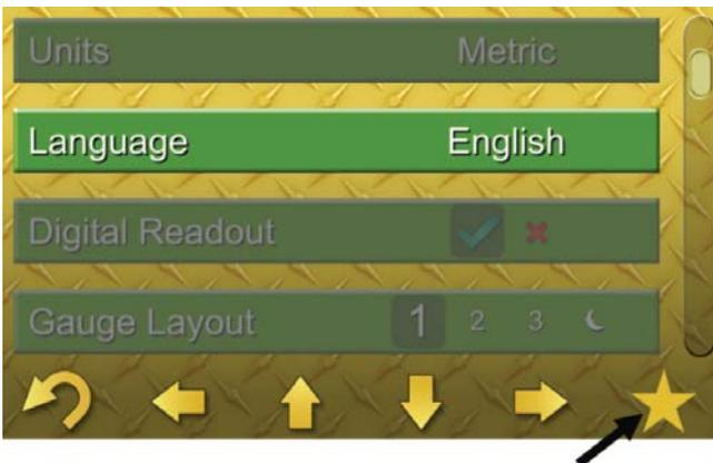
When a “Favorite” is established, a solid star icon will appear above one of the soft keys anytime the main monitoring screen is the active display. Pressing this soft key will immediately jump the user to the sub menu where the “Favorite” setting is located and highlight the setting.
