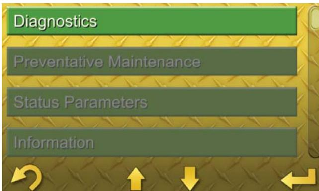
The screens within this sub menu allow the user to view active (currently occurring) or logged (having occurred; may be active or no longer active) machine condition warnings.
