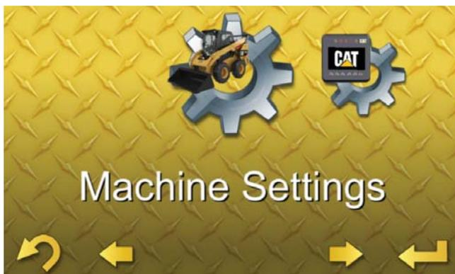
The “Machine Settings” menu allows the operator to adjust several machine response and performance settings. These settings will be stored under each operator profile. When the Anti-Theft Security System is enabled, the settings take effect each time an Operator Code is entered at the log in prompt. If the Anti-Theft Security System is not enabled, the operator settings at the time of the previous KEY OFF will remain in effect. See “Anti-Theft Security System.”
