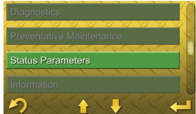
The “Status Parameters” screen shows the status of some of the most important machine parameters such as throttle position, engine speed, joystick position, battery voltage, and drive motor speed. The parameter status information may be useful for basic troubleshooting.
