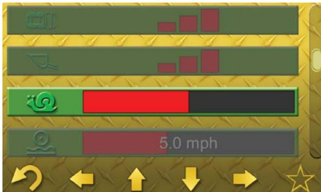
The “Creep Control” mode allows the operator to set a maximum machine travel speed at full joystick movement. Use Creep Control for operations that require slow, constant speed independent of engine idle speed, such as cold planning or trenching.
