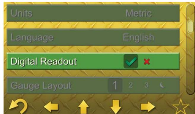
The “Digital Readout” allows the operator to either have the numerical gauge values display turned ON or OFF. The factory default is “ON.”
