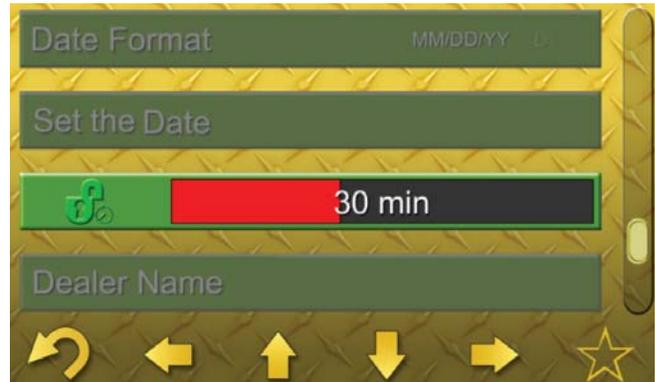
If Machine Security is enabled, the “Security Grace Period Adjustment” allows the user to select from several choices of grace periods, which will determine how long the machine remains unsecured once Keyed OFF. The grace period timer begins at Key OFF and during the grace period, the machine will not require reentry of a PIN when Keyed ON again.
