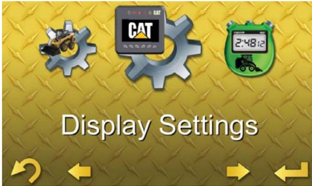
The “Display Settings” menu allows the operator to adjust several aspects regarding the look of the display. These adjustments will be stored under each operator profile. When the Anti-Theft Security System is enabled, the settings take effect each time an Operator Code is entered at the log in prompt. If the Anti-Theft Security System is not enabled, the operator settings at the time of the previous KEY OFF will remain in effect. See “Anti-Theft Security System.”
