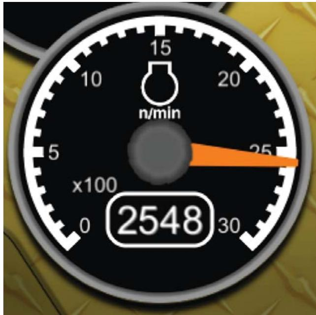
The needle indicates the engine's RPM. If the gauge's numerical values are enabled, the background will change from black to red to indicate that the engine speed is above the allowable HIGH IDLE limit. The throttle should be turned down to the acceptable range. The Cat dealer should be contacted to determine the cause. See "Display Settings, Digital Readout."
