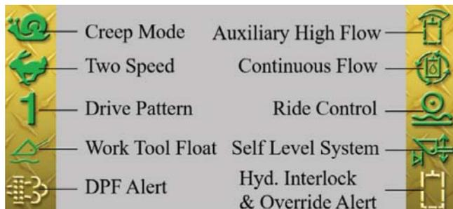
There are several alert indicator icons located along the sides of the display window and will activate as needed. See the machine's Operation and Maintenance Manual "Alert Indicators" for a description of the warnings and mode indicators.
