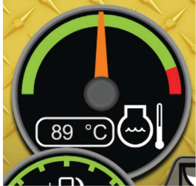
The needle in the red zone indicates that the engine coolant temperature is too high. If the gauge's numerical values are enabled, the background will change from black to red to indicate that the engine coolant is approaching an unsafe temperature. The machine should be stopped soon and the engine set to low idle to allow the engine to cool. See “Display Settings, Digital Readout.”
