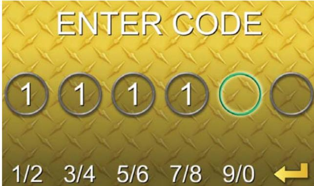
The default Master Code is “1111” and is established when the Anti-Theft Security System is first enabled. This code should be changed by the owner as soon as possible as a security best practice. Options available in the User Management menu while logged in under the Master Code are as follows:
