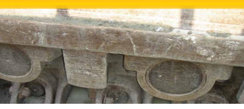
"6060 HD rollers: 9,000 hours and still going." A customer in South Africa was unsatisfied with the performance of legacy 6060 rollers—whether they were from Caterpillar or competitive aftermarket offerings. The legacy rollers would fail by overheating or breaking the center weld in as little as 80 hours and had a maximum life of 8,000 hours.
