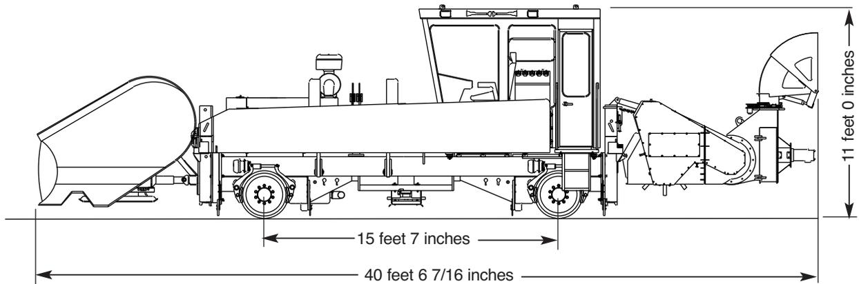
**Description:** Kershaw 60-2 Snow Fighter is equipped with a 10 ft. V-type snow plow, benching-type snow wings and a broom/snow switch cleaner attachment for snow removal from the track area. With the addition of the optional Snow Switch Cleaner, snow can be removed from switches and propelled clear of the track.
