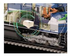
A single EMD lithium ion battery replaces two traditional lead-acid batteries on a locomotive.
