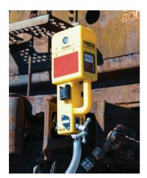
End-Of-Train (EOT) devices transmit real-time, vital information from the end of the train to the locomotive cab.
