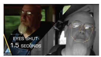
The underlying Driver Safety System (DSS) technology is based on patented eye-tracking and analytics that detects driver distraction and fatigue while on the job.
