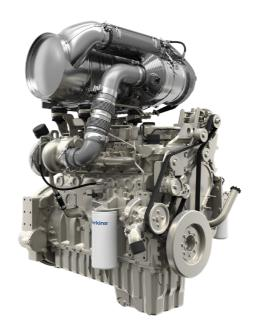
The **1706J** is a six cylinder 9.3 litre unit that delivers an industry-leading maximum power rating of 340 kW (456 hp) and meets EU Stage V and U.S. EPA Tier 4 Final emissions standards. Recent advances include an updated common rail fuel system, simplified aftertreatment and removal of exhaust gas recirculation (EGR).
