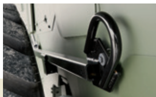
Removable bracket for C-130 air transport.
