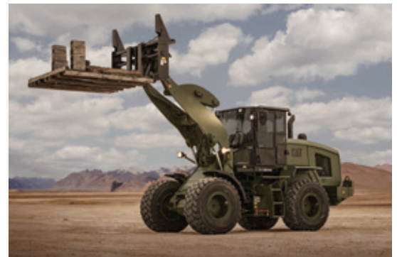
930K ADL with hydraulic adjustable forks.
