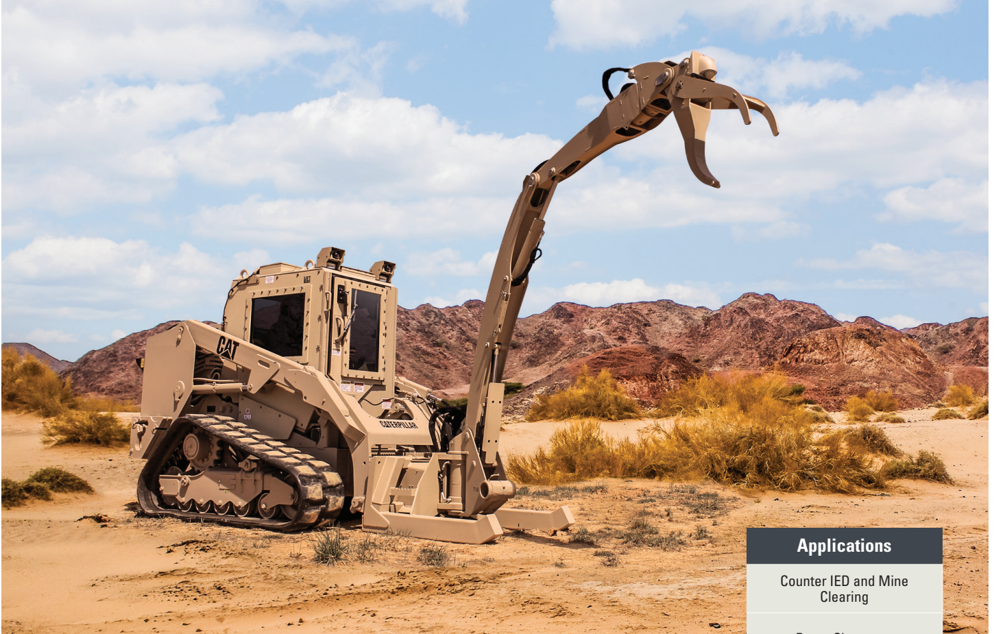
Armored 279D3 Compact Track Loader (CTL) with boom and grapple arm.
