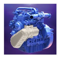
**Hybrid-hydraulic**: Stores excess energy from the engine, and recovered energy from machine systems, in a hydraulic accumulator. Offers rapid release of stored energy and leverages existing machine hydraulics. Service network friendly.
