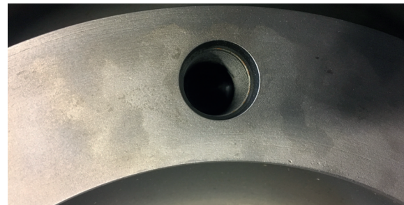
Main contact surface with insufficient reconditioning.
