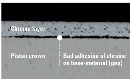
Cross section of ring groove flank with bad adhesion of chrome layer.
