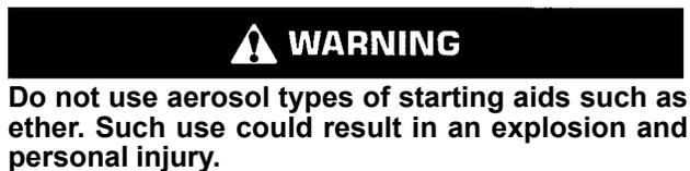
**Do not use aerosol types of starting aids such as ether. Such use could result in an explosion and personal injury.**
