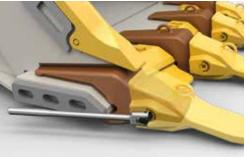
Turn retainer 180° counterclockwise to unlock.
