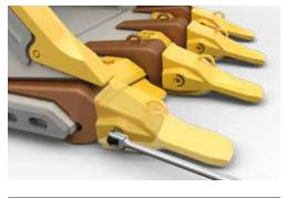
Wider top surface reduces drag on the tip and adapter side as the tip moves through the soil. Reduced side drag results in less force required to move the bucket through the soil.
