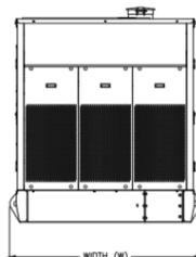
Sound Attenuated & Weather Protective Enclosure on Skid Base
