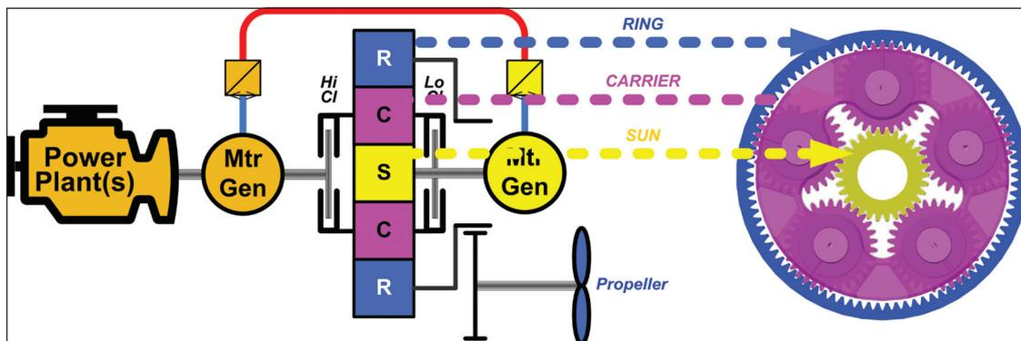
Figure 5: AVD propulsion system diagram
