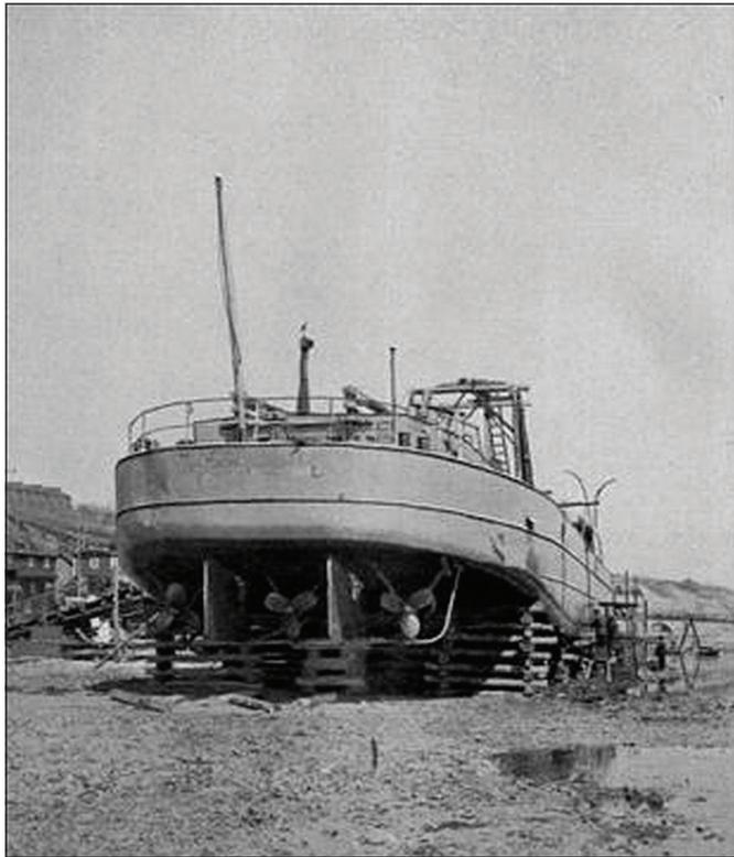
Figure 1: Stern view of the oil tanker **Vandal**, showcasing triple propeller arrangement
