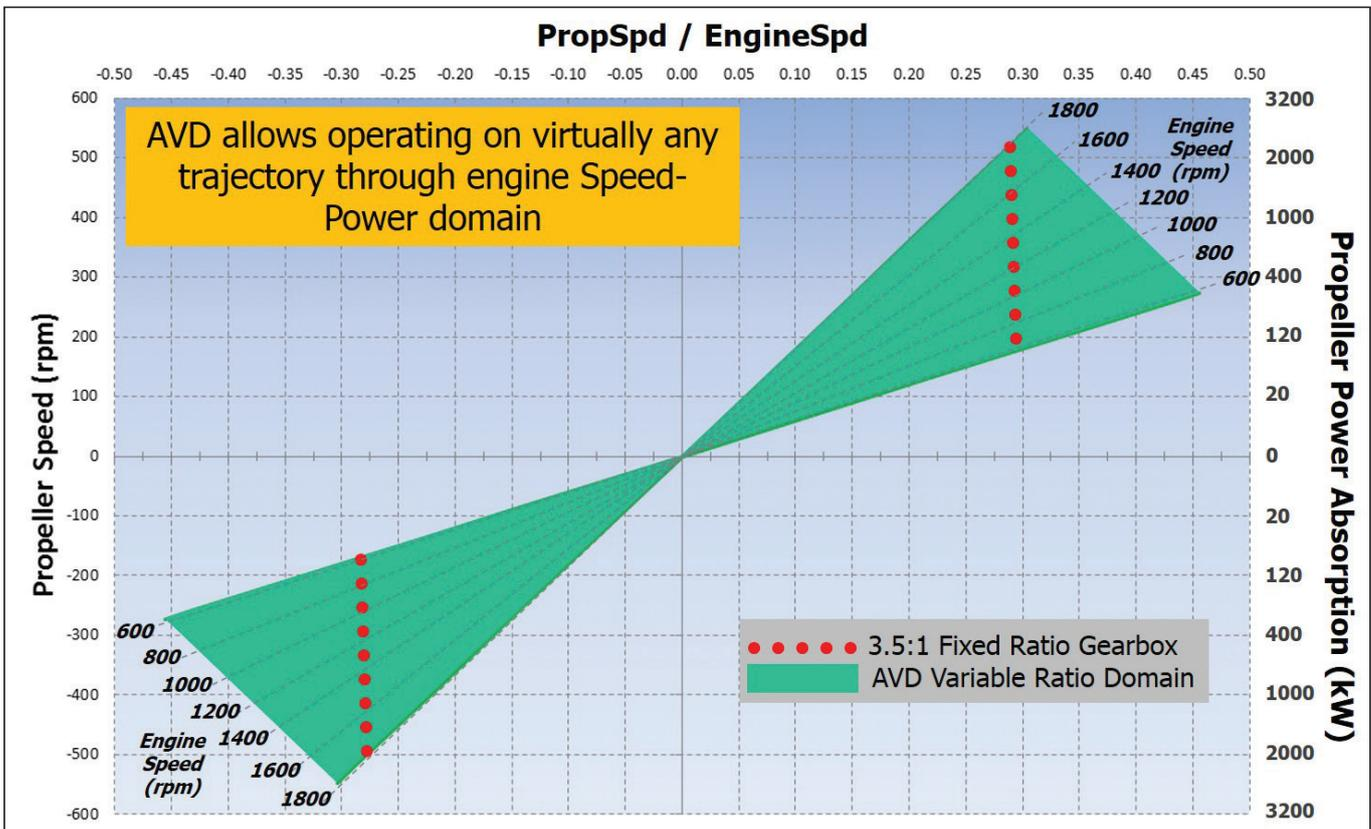
Figure 11: Ratio range domain of a fully reversing 2.5MW AVD propulsion system with fixed ratio gearbox reference
