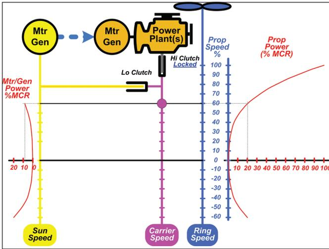
Figure 8: The AVD Variator mode to Variator-Mechanical mode shift
