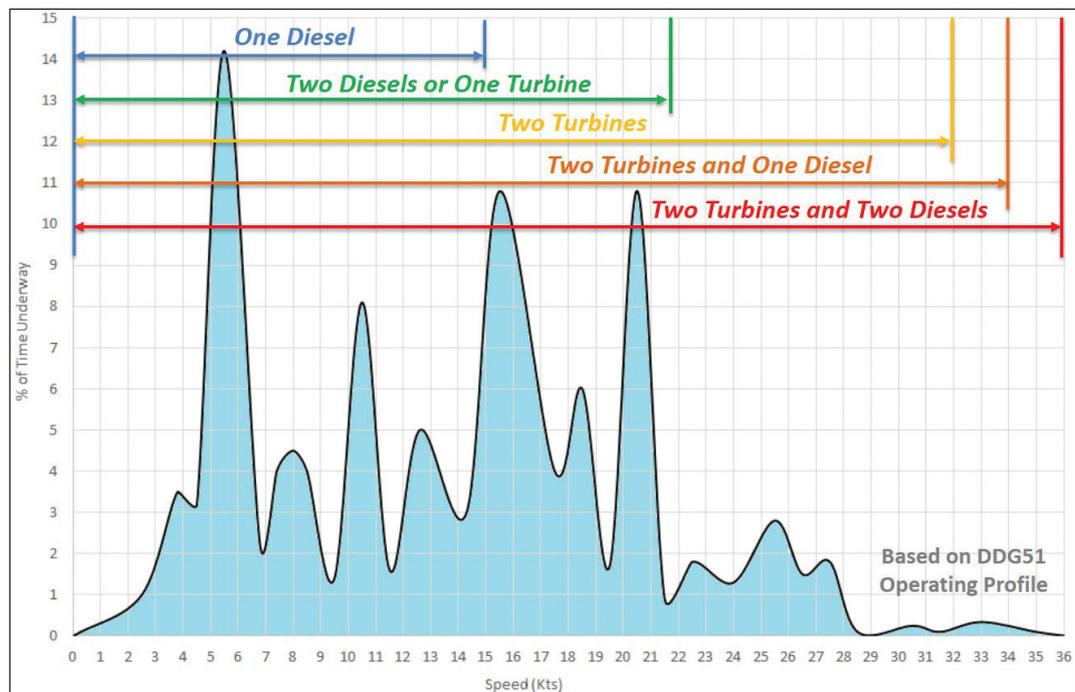
Figure 23: AVD-equipped small surface combatant vessel performance in normal propulsion modes
