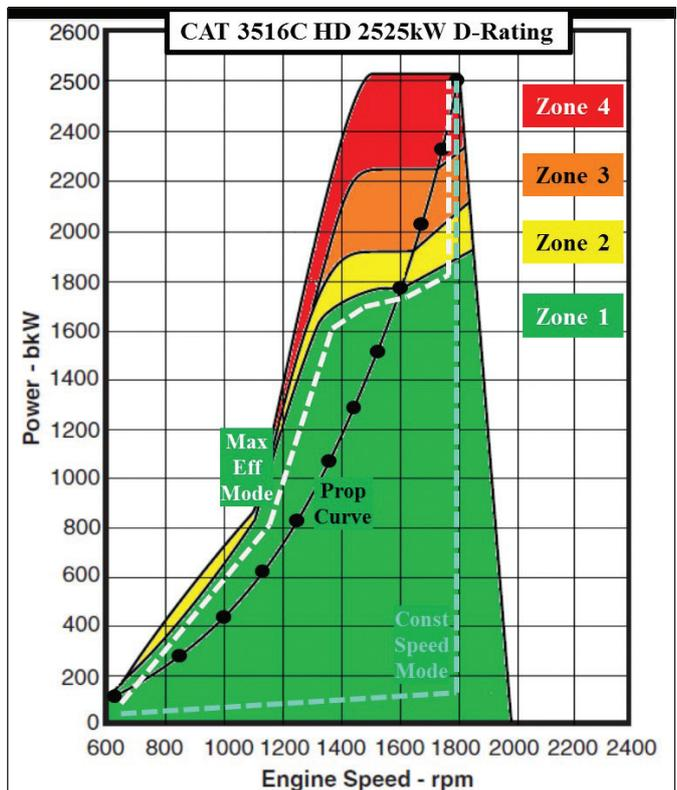
Figure 12: Examples of AVD operating trajectories plotted on an engine speed-power envelope
