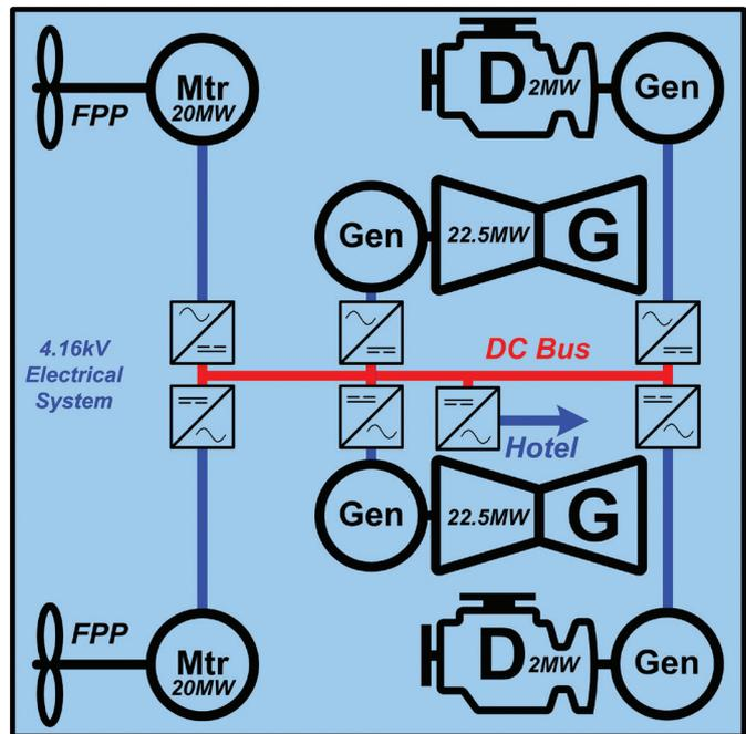
Figure 19: Simplified Type 45 destroyer integrated electric propulsion diagram
