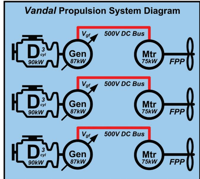
Figure 3: **Vandal** propulsion system diagram
