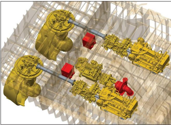
Figure 17: An AVD propulsion system installation in a harbour tug
