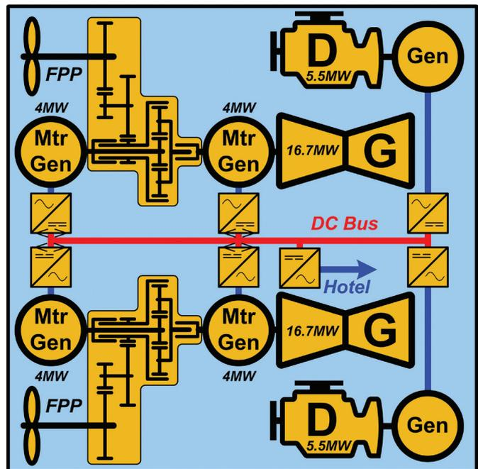
Figure 20: Simplified AVD propulsion system diagram for a small surface combatant vessel
