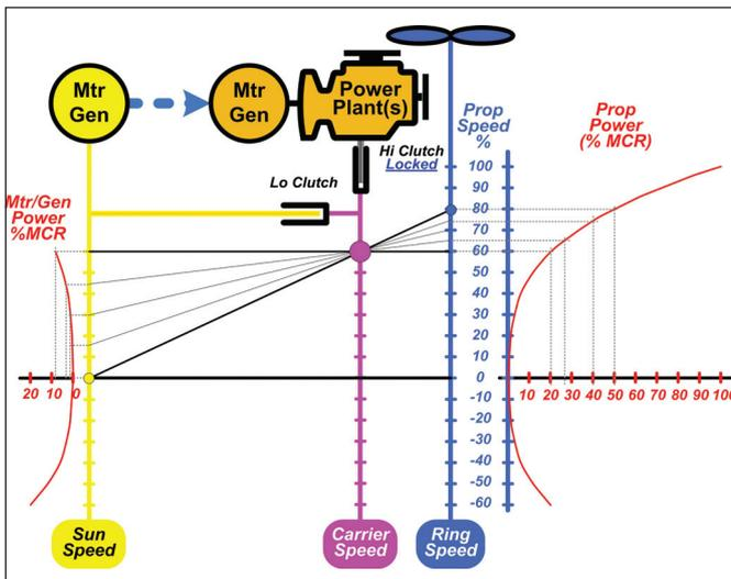
Figure 9: Regenerative portion of the AVD Variator-Mechanical mode
