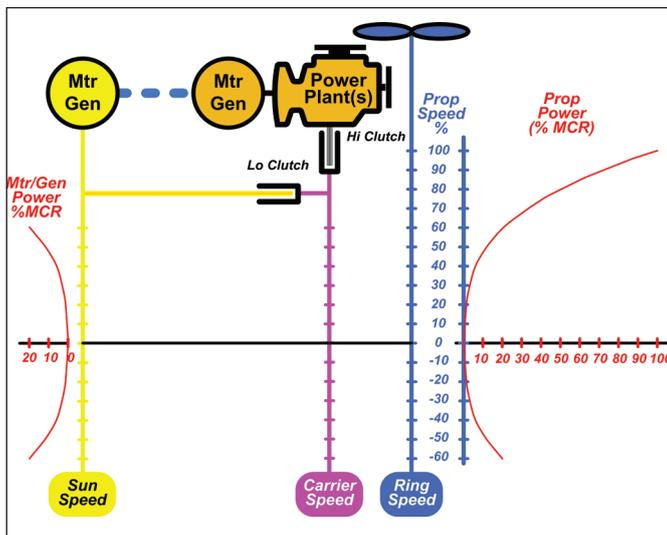
Figure 6: Graphical representation of the AVD speed-power relationships
