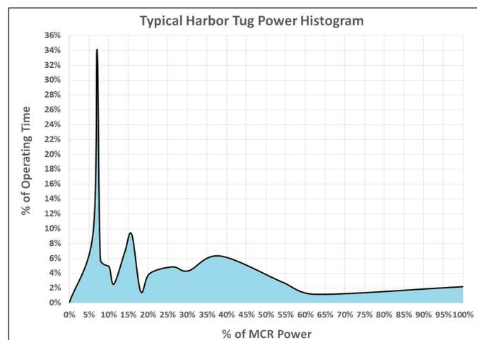
Figure 16: A typical harbour tug power histogram
