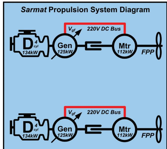
Figure 4: **Sarmat** propulsion system diagram
