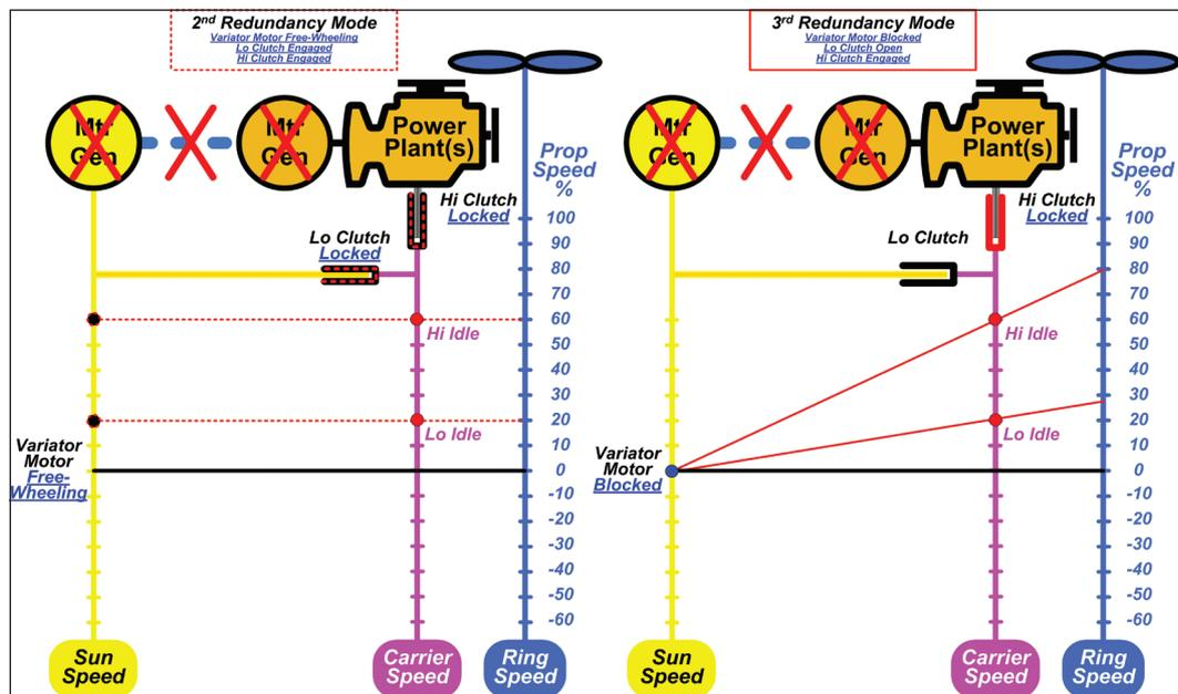
Figure 15: AVD mechanical redundancy modes
