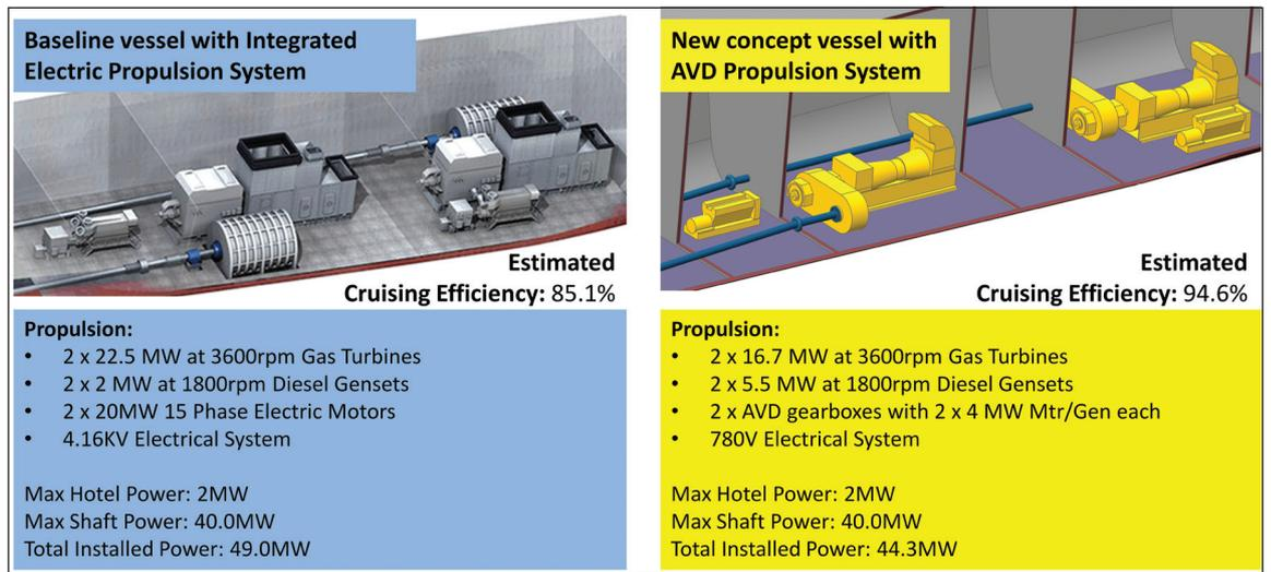
Figure 21: Packaging comparison between IEP and AVD
