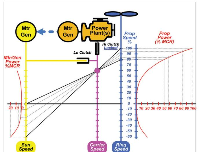
Figure 10: The additive portion of the AVD Variator-Mechanical mode
