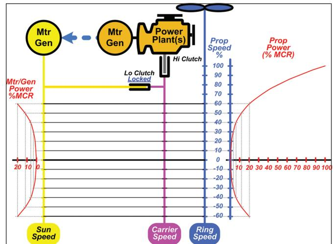
Figure 7: The AVD Variator mode of operation
